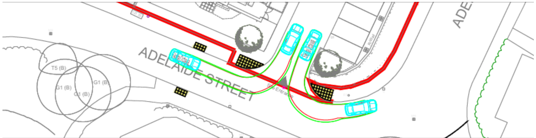
SITE ACCESS TWO-WAY VEHICLE TRACKING (1:250)
